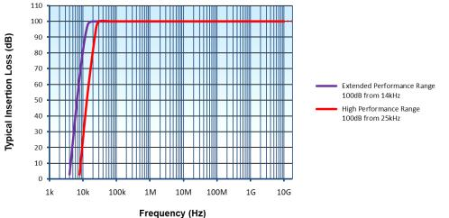
Asymmetric Performance in 50Ω System With or Without Load
